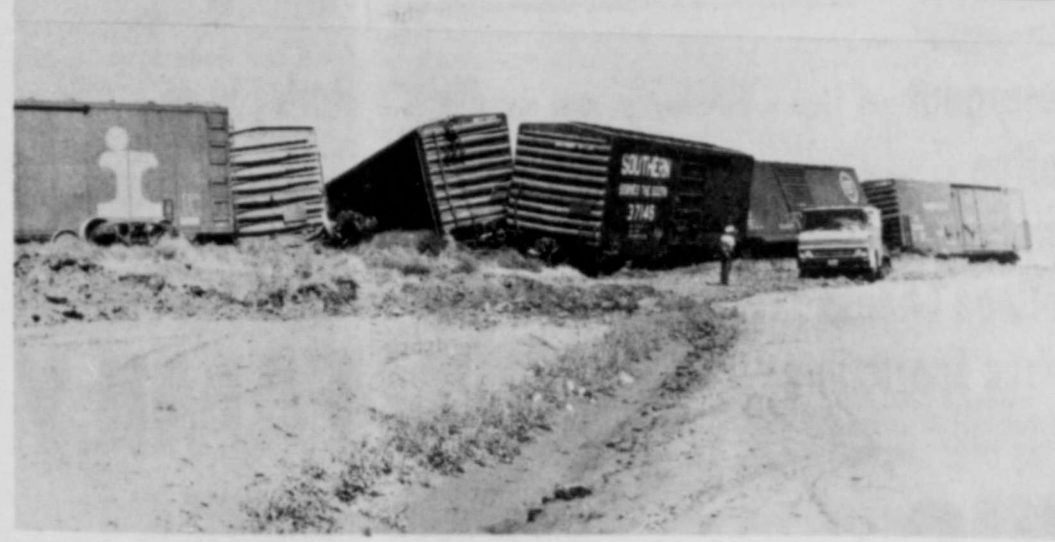
A BROKEN RAIL caused the derailment and damage to nine loaded freight cars for Fort Worth and Denver early Friday morning on the line between Barwise and Petersburg. The engine stayed on the track. Workmen are pictured busily rebuilding the track. (Staff Photo)
