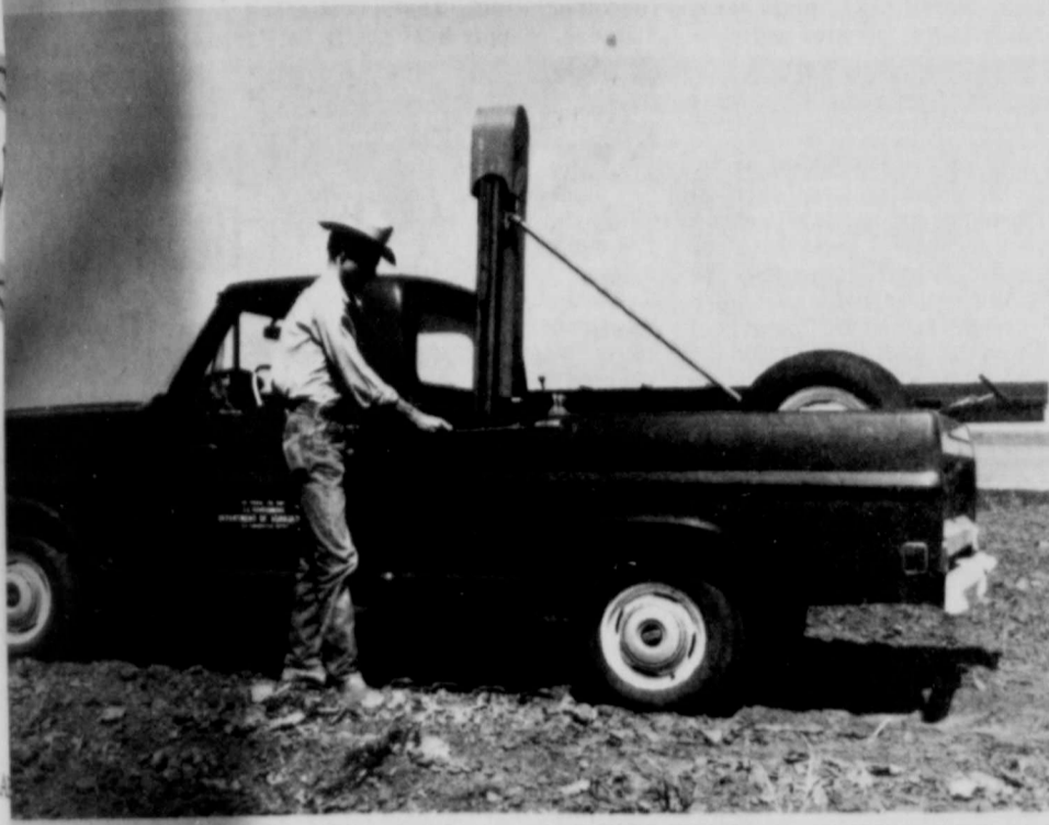
ED ABOVE is Conrad Neitsch, Soil Scientist with the Soil Conservation Service, examining a soil profile by use of a hydraulic probe. The probe, which can reach depths of 8 feet, speeds up the soil sur- (USDA-Soil Conservation Service Photo)
