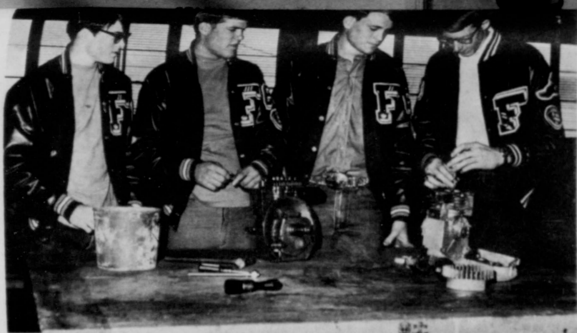
SHOP PROJECT-GASOLINE ENGINES. . . (left to right) Bob Marler, Jody James, and George Quisenberry look on as Joe Thurston places a piston in a small gasoline engine in the Ag Shop. (Staff Photo)
