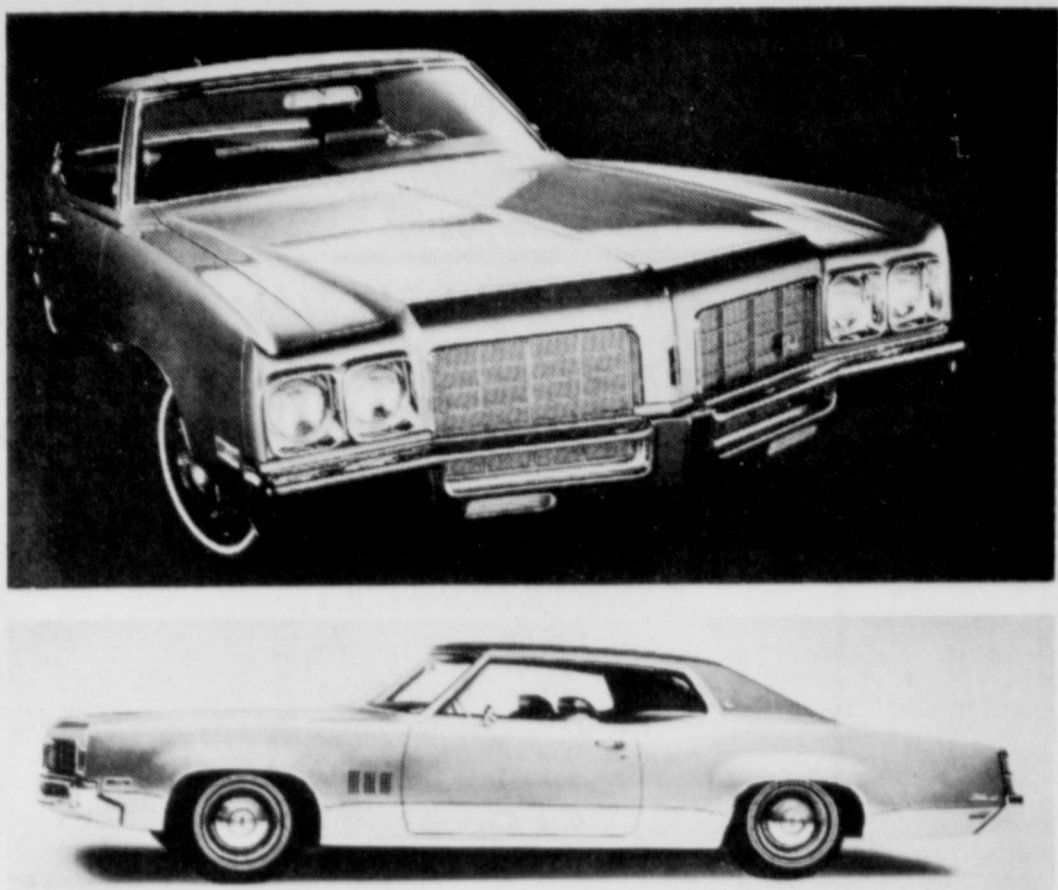
Offered exclusively in a Holiday Coupe body style, the 1970 Delta 88 Royale represents the top of Oldsmobile's '88' line of cars. A vinyl-covered top, distinctive grille, front fender louvers and specific exterior ornamentation easily identify the Delta 88 Royale. Standard engine on this 1970 Oldsmobile is a 455-cu.-in. V-8. A high output engine option, designated W-33, is available on the Delta 88 Royale and on all other Oldsmobile '88' models for 1970.
