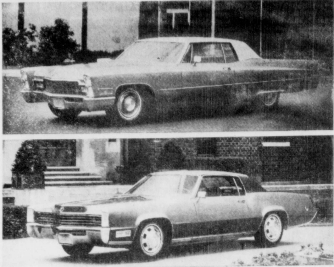
Exterior changes in the 1968 Cadillac, as shown on this Coupe de Ville (top), include a new grille and larger parking lights redesigned cornering lights and new marker lights on the side plus a new deck lid and all chrome rear bumper. Among the safety related product improvements in all models are: a new concealed windshield wiper and washer system, recessed door handles and added cushioning in the instrument panel and front seat backs. Dramatic styling changes to Cadillac's 1968 Fleetwood Eldorado (bottom) include new parking lamps located in the leading edge of the front fenders, a new hood 4 1/2 inches longer and redesigned taillights. All 1968 Cadillac models are powered by a new 375 h.p. — 472 cubic inch engine which produces 525 foot pounds of torque — the highest of any production passenger car engine in the world.
