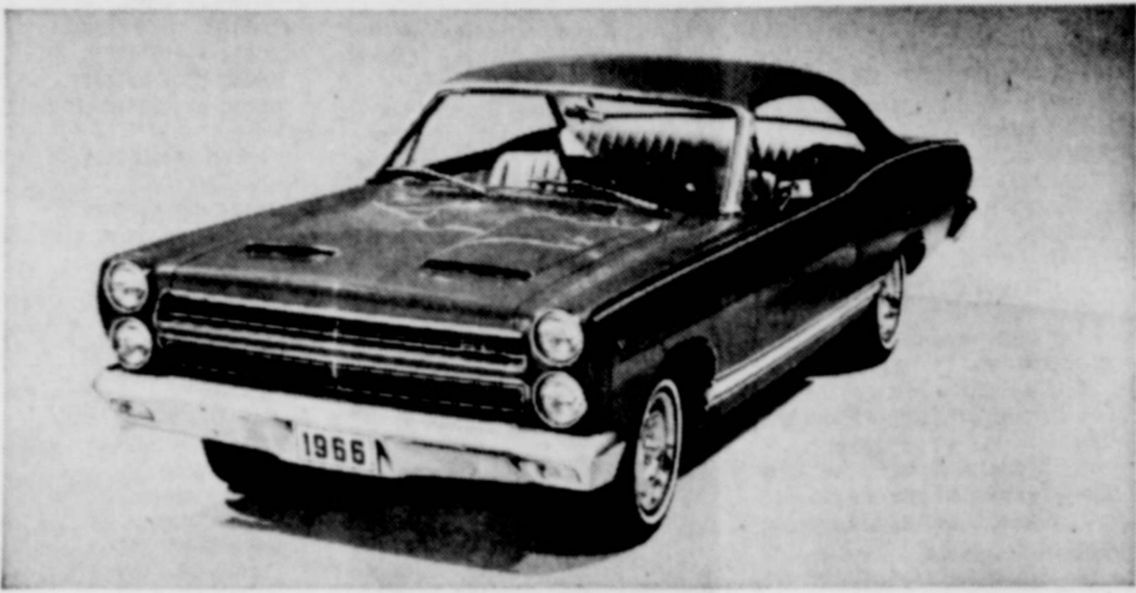
Completely restyled for 1966, Comet features a new larger body, a host of luxury appointments and a wider choice of engines. Overall length has been increased by eight inches and wheelbase is two inches greater at 116 inches. Two Mercury 390-cubic-inch engines are added to the power offerings. Sportiest of the new Comets is the Cyclone GT model (above) which offers a high performance 335-horsepower V-8 engine and a unique fiberglass hood with simulated air scoops. The 1966 Comet goes on sale October 1.
