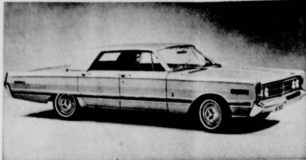
Mercury for 1966 again moves forward as a premium car in the medium-price field with tasteful styling changes, new engines and important additions to the option list, including disc brakes. Standard in top-of-the-line Park Lane series (above) and optional in other Mercurys is an exclusive new 410-cubic-inch 330-horsepower engine. The new Mercurys will go on sale in dealer showrooms October 1.
