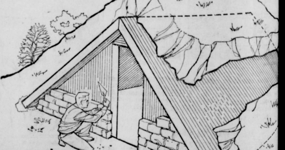
LEAN-TO SHELTER made of lumber would provide protection against fallout in homes with basements, costing less than $75 on a self-built basis, would provide protection as some of the seven other designs in the Defense Department's booklet, "Family Shelter Designs." It combines simplicity of construction, availability of materials, and could be disassembled. Defense offices have the free booklet available now.
