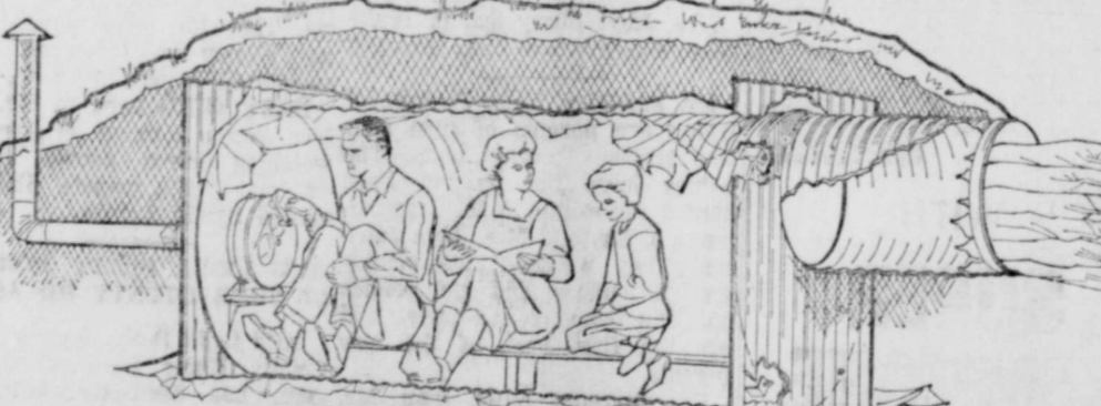
PRE-FAB corrugated steel culvert fallout shelter for three persons can be bought for about $150, plus delivery and installation. The shelter, which would cut to 1/500th the amount of outside fallout radiation exposure of its occupants, is included in the "Family Shelter Designs" booklet now available at state and local civil defense offices for public distribution. It is available without charge.
