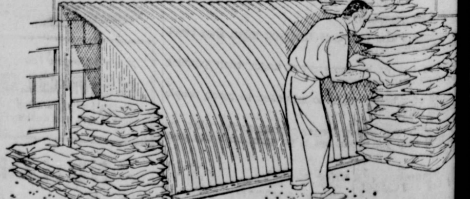
ABOVE-GROUND SHELTER covered with earth for areas where basements or underground construction are not feasible would provide good fallout protection for up to 10 persons. The shelter, costing $550 for materials, is one of the "Family Shelter Designs" booklets available from the Department of Defense, and available at no charge through civil defense offices.
