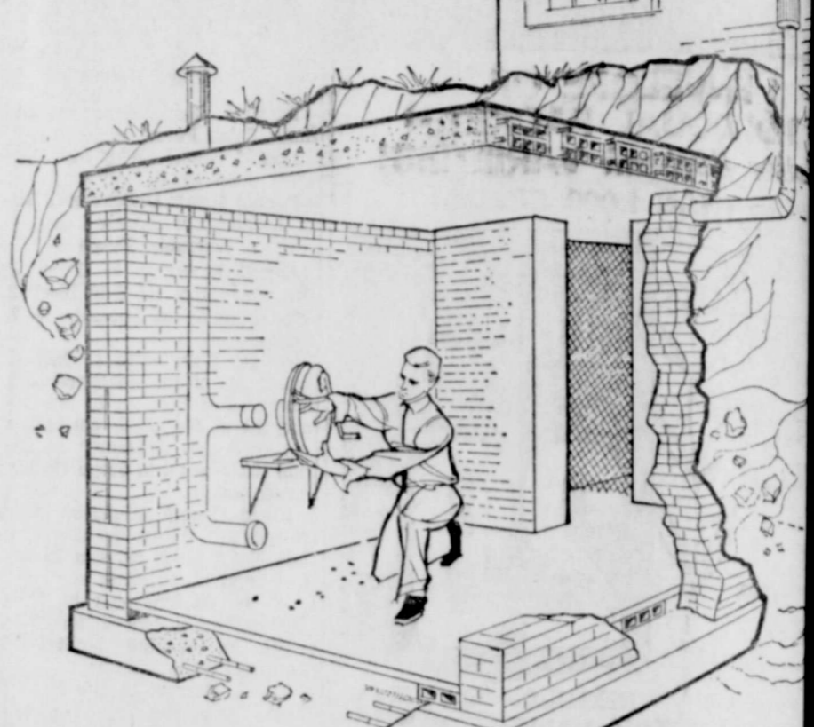
DUAL-PURPOSE underground fallout shelter of clay masonry construction and designed to be built as part of new house would combine some nuclear blast protection, excellent shielding from fallout, and the usefulness of an ordinary basement.
