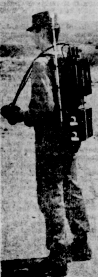
Soldier at Fort Huachuca, Ariz., with lightweight radar unit that is carried on the back. Goal of Signal Corps experimenters is completely mobile detection unit.
