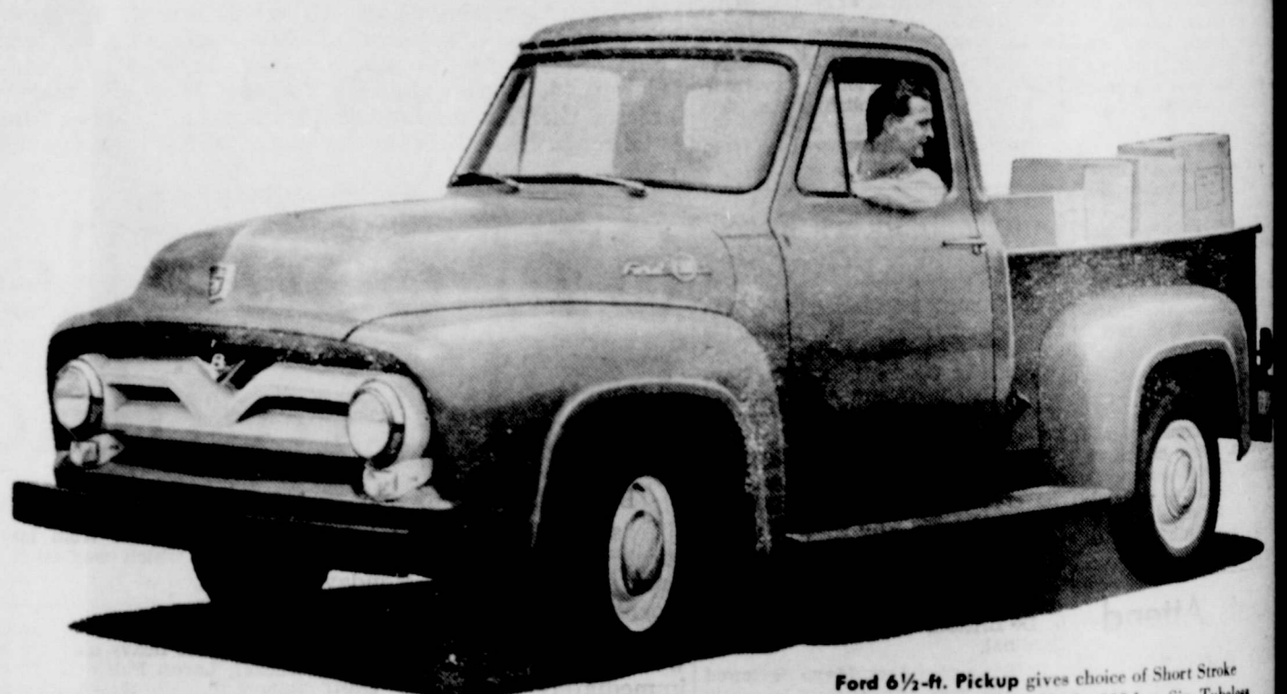
Ford 6 1/2-ton Pickup gives choice of Short Stroke 132-h.p. V-8 or Short Stroke 118-h.p. Six. Tubesteer tires standard. Fordomatic Drive and Power Brakes available at low extra cost. GVW 5,000 lbs.
