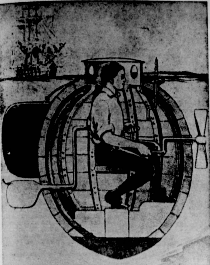
19TH CENTURY SUBMARINE: David Bushnell's "Marine Turtle," which attacked the British frigate HMS Eagle in New York Bay in 1776, but failed in her efforts to fasten a mine to the ship's copper sheathed bottom. This was the first American submersible.
