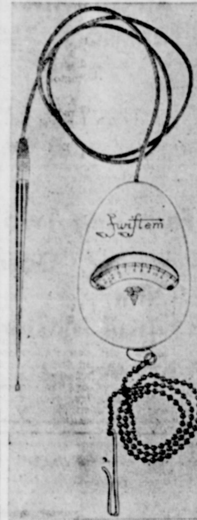
ELECTRONIC thermometer developed by Army dentist is easy to read, won't break and gives accurate reading in five seconds.
