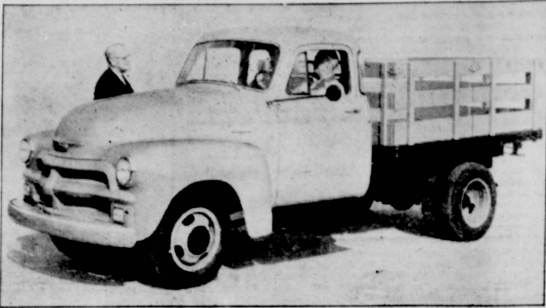
Typical of completely re-engineered Chevrolet trucks making their 1954 model debut at dealer showrooms this week is the three-quarter ton (6500 GVW) stake, on which dual rear wheels are now available. Loading height has been lowered
