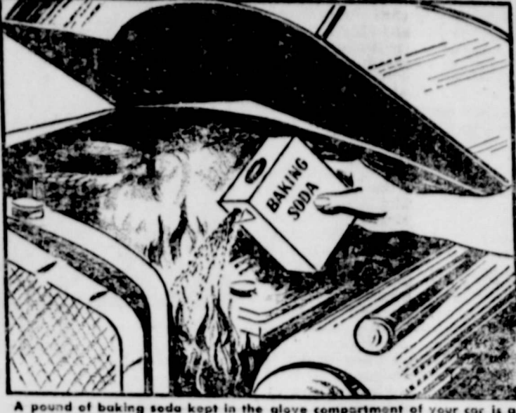
A pound of baking soda kept in the glove compartment of your car is a wise precaution. Fires can get started quickly — in the engine, even in the upholstery or ashtray. Sprinkle soda over the smoking spot, and fire will be instantly extinguished. Baking soda produces carbon dioxide which settles around the blaze, cuts off its oxygen, and quenches the fire.
