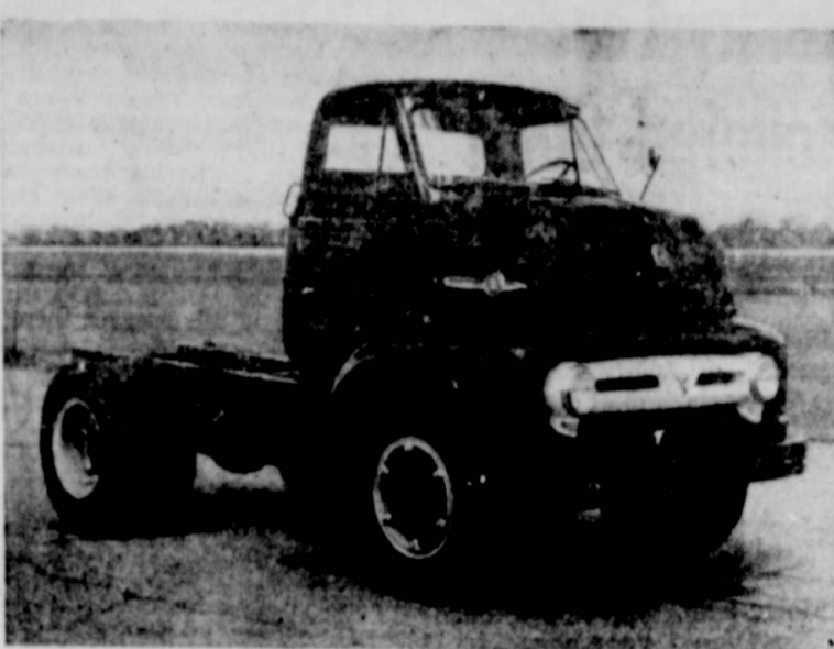
Ford engineers claim these newly-designed C-750 Series cab forward trucks set a pattern for the industry with their wider, 3-man cabs with full-width seats. They have greater maneuverability and shorter turning radius; new, curved, one-piece windshield with 55 percent more visibility and 4-foot wide rear window. Synchro-silent transmissions do away with double clutching. This new cab-forward design makes possible almost all engine service operations from the front of the truck.
