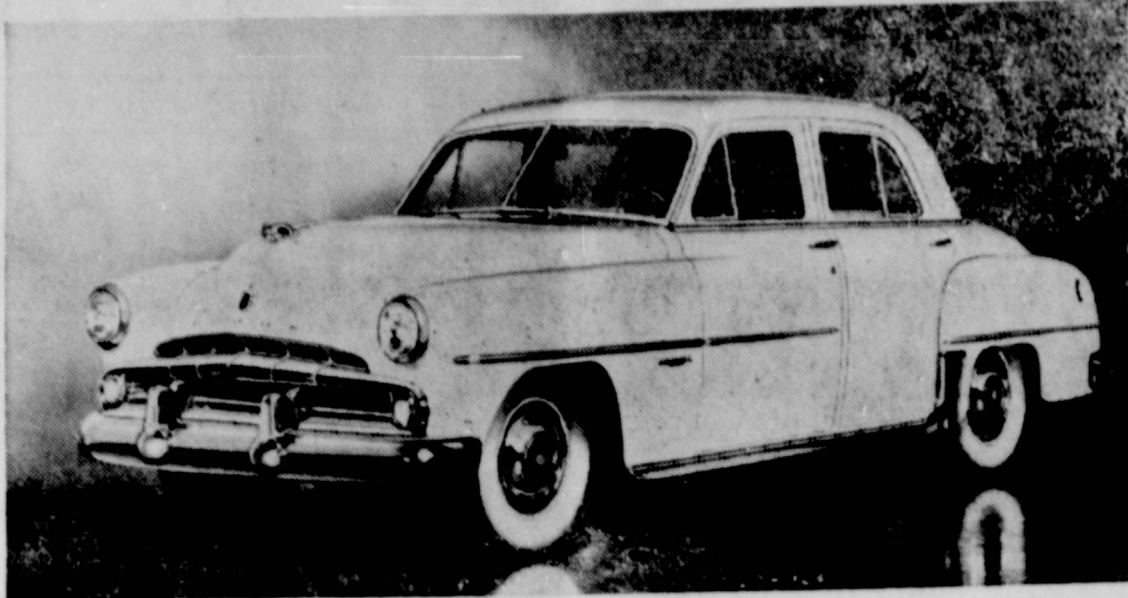
The 1951 Dodge Coronet four-door sedan has a wider windshield and wider rear window for improved driver vision. Bumpers and bumper guards are larger and the grille and hood are of a new modern design. All 1951 Dodge cars are equipped with the new, more comfortable riding Oriflow shock absorbers. The model shown above is available with Gyro-Matic shift-free transmission.
