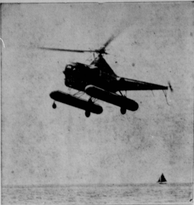
RESCUE SHIP OVER LAND OR SEA—With its new wheels prominently displayed, the Air Force's first amphibious helicopter, the H-5H, is shown making a routine over-water flight. The wheel-boat combination greatly increases the H-5H's utility as a rescue, search and liaison aircraft, allowing it to land with equal facility on land or water.
