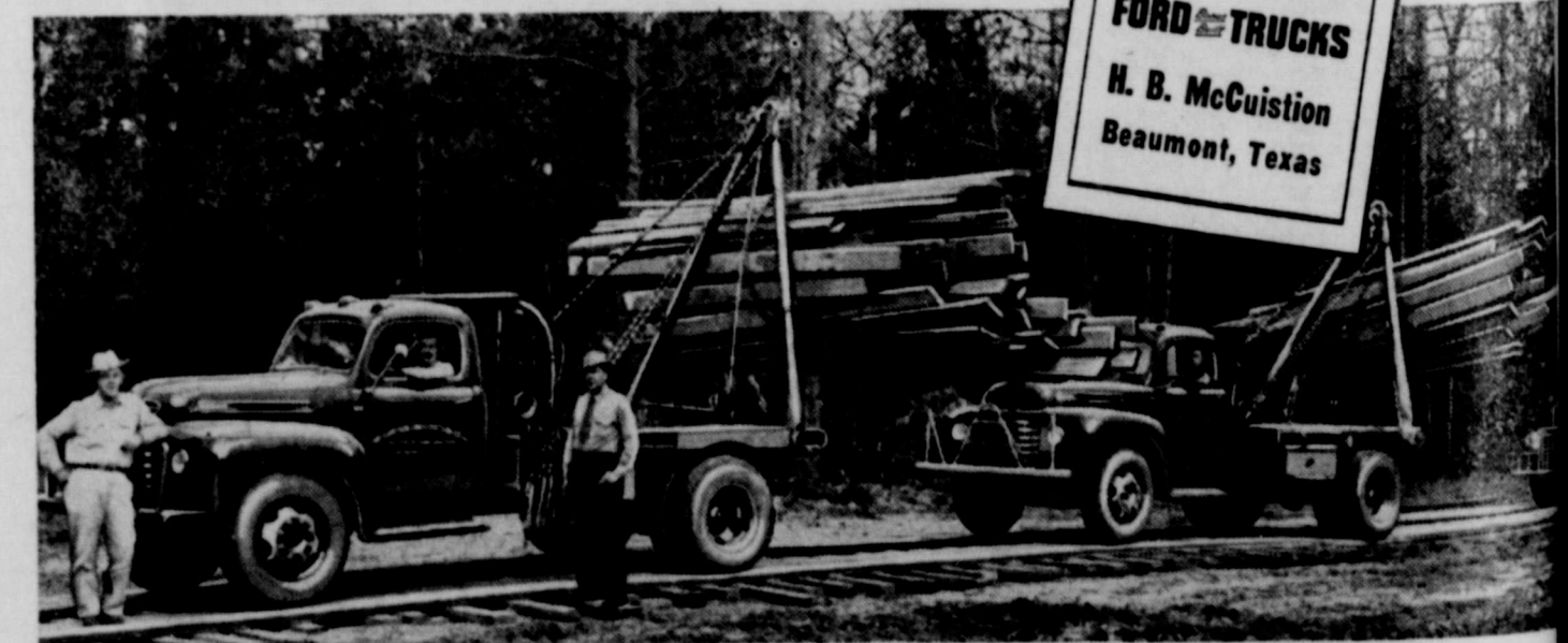
Ford Model F-7 Big Job shown has Gross Vehicle Weight rating of 19,000 lbs.; Gross Combination Weight rating of 35,000 lbs. as shown.
