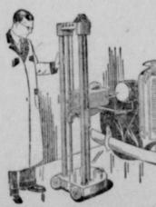
FAULTY HEADLIGHTS are one of the Chief Causes of Highway Accident. Road way Bumps and Jars make adjustment necessary at least twice a year.
