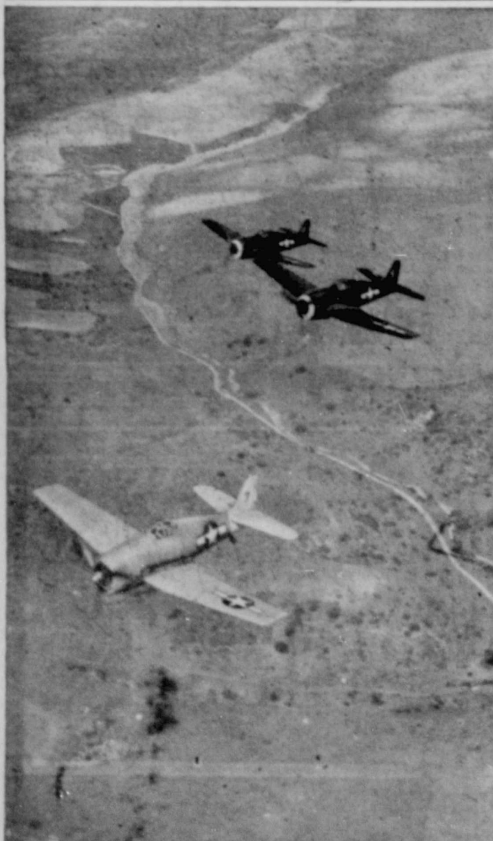
Called by two "mother" planes, a pilotless Navy Helicat (Grumman FC7) sails over the San Diego area in a dress rehearsal for similar air data operations planned as part of the atomic bomb tests at Bikini atoll this summer. The drone (foreground) is controlled by the "mother" Helicat immediately behind it. The rear plane serves as standby should the first one fail. During the tests four drones, each with two control planes, will be launched from the USS Shangri-la and will be controlled first from the carrier's deck, then from a mother plane in the air and finally from the ground control operator on Rot Island where they will land. (Joint Army-Navy Task Force)
