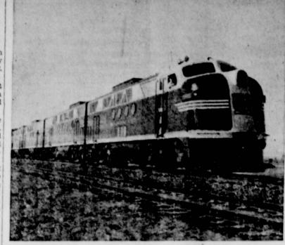
World's first diesel freight locomotive has just been placed into service by Santa Fe. The powerful engine made its first regular run over the lines on February 6. The locomotive is field Sunday after visiting with her 193 feet in length and is divided into four sections so as to permit curve rounding. Several thousand persons viewed the initial run of the new locomotive.
