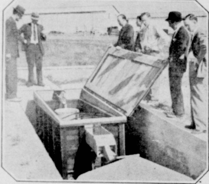
Measurement of soil and water losses is an important part of the Dixon Springs conservation experiment. Here is the device for such measuring being inspected by workers at the experimental station.
