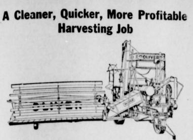
An Oliver Combine will do a quicker, cleaner, more profitable harvesting job for you. There is a size for every need and the 10 and 12-foot machines are proving especially popular. The header is braced and trussed into a practically complete unit. It is hinged to follow the contour of the ground and cut clean up-hill, down-hill or on the level.
