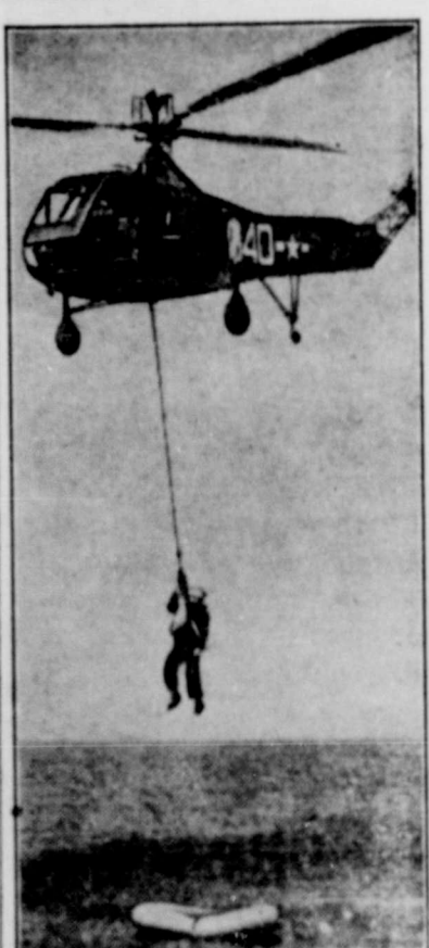
One of the first test pickups from a rubber life raft that proved the success of the Vickers hydraulic hoist. Commander Erickson is piloting the helicopter.
