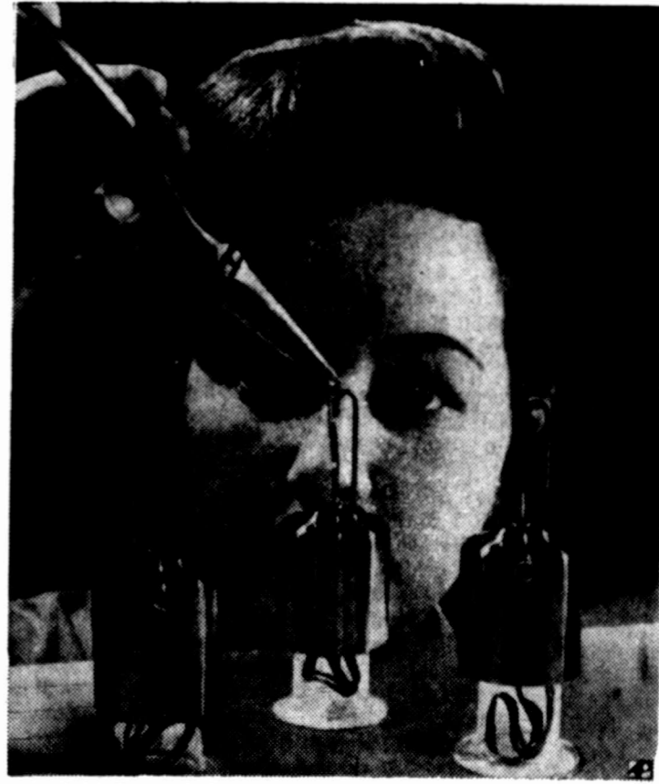
TOUCH CONTROL — Worker guides a tungsten filament of 125,000-volt x-ray valve tube for attachment to a cathode support during assembly at Bellwood, Ill., plant.
