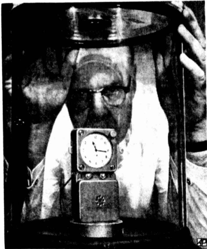
CHECKOUT — Alarm clock for use by astronauts aboard the first U.S. manned space station is prepared for vacuum and temperature tests at Bulova plant in New York.
