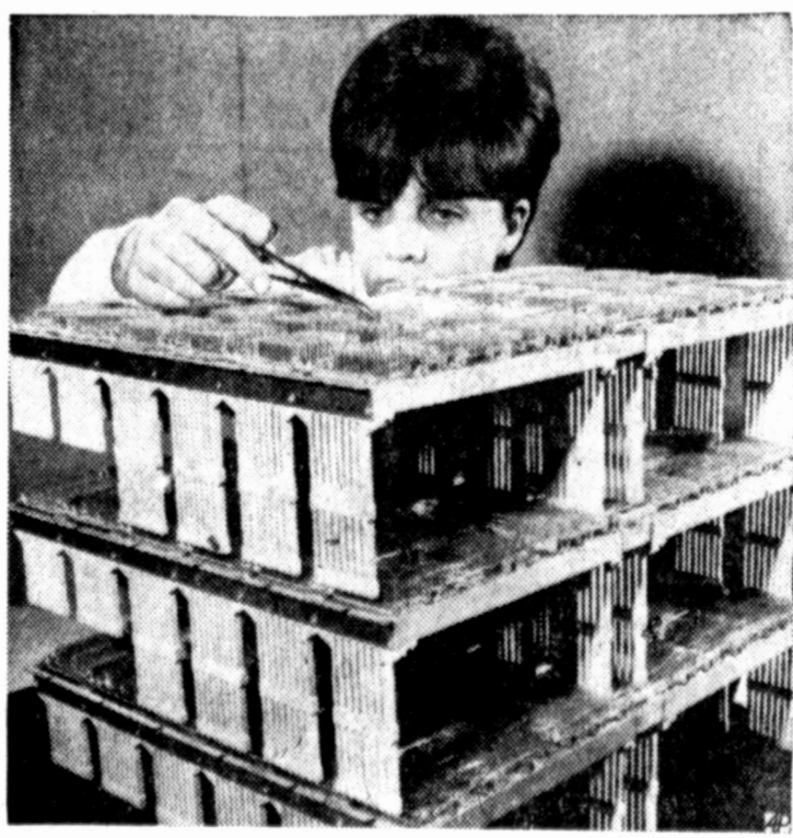
WORD LIBRARY — Technician works on stack of integrated circuit core memories at Honeywell plant in Framingham, Mass. Each section adds to computer's memory.
