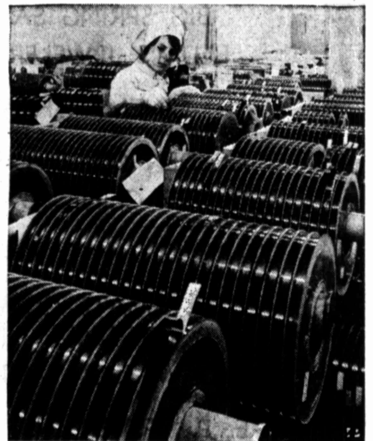
TAPE POOL — Magnetic tape is checked and tabbed at Indianapolis plant. Each spool is capable of storing up to 46 million bits of computerized information.
