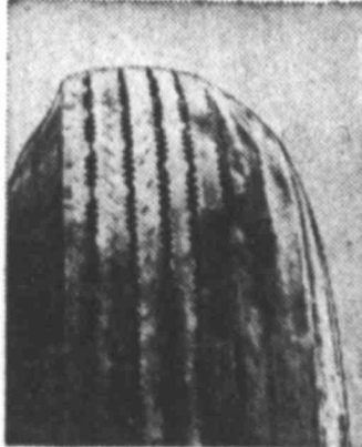
Tire shows extremely uneven wear. It means: (1) faulty brake system (needs fluid, adjustment) (2) faulty wheel alignment (too much camber) (3) tires need rotation (including spare)
