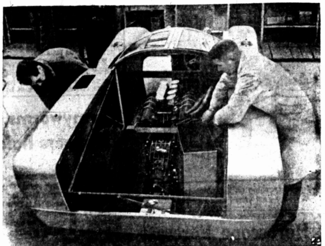
WHEELS OF PROGRESS — Mechanics work on the body and V8 engine of 200 mile per hour Healey two litre sports racing car at the Donald Healey works at Warwick, England.
