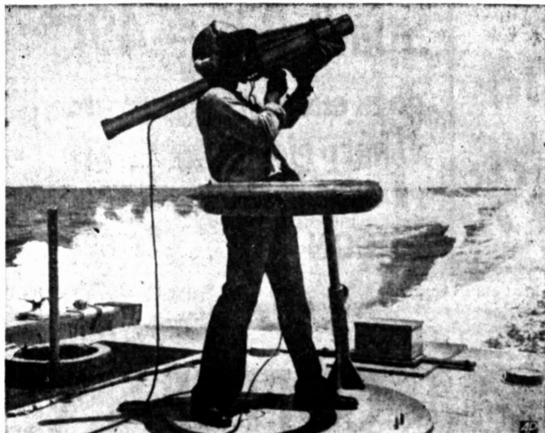
READY ON FIRING LINE — A Redeye missile, designed to strike low-flying aircraft, is tested for shipboard use on the Pacific Missile Range off Point Mugu, Calif.
