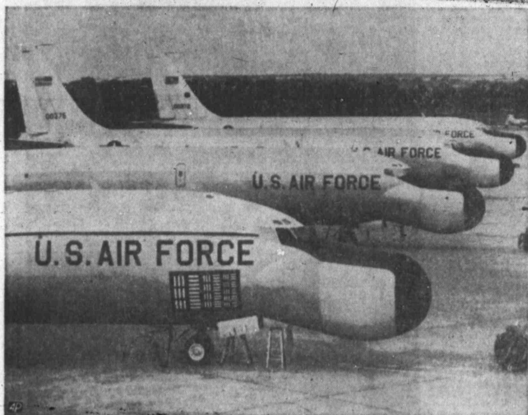
SHAPED FOR SPACE —The unusual noses of these U.S. Air Force 40-136M jets at Tulsa, Okla., are radomes housing antennas. They're used to track a spacecraft and lock onto it for transmission and reception of voice and telemetry communications.
