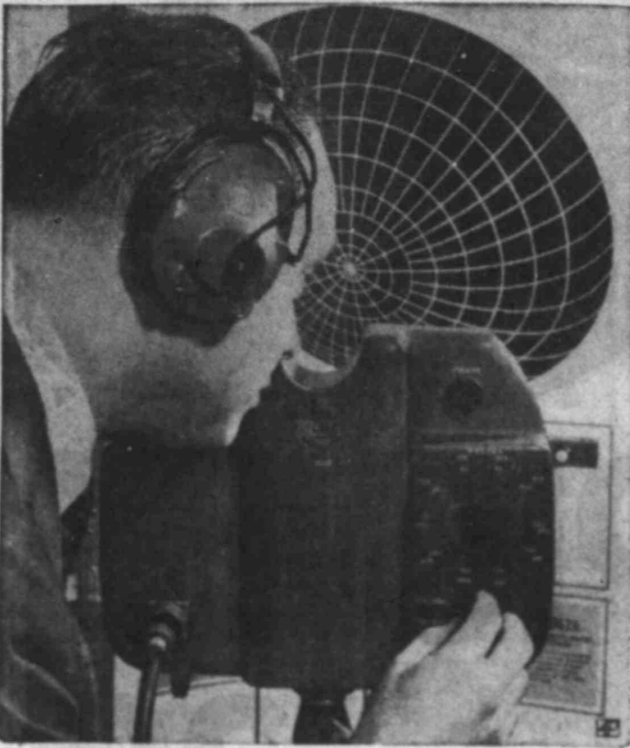
COMBAT AID —RCA engineer demonstrates 2-pound radar designed to enable infantrymen to detect man-sized targets, despite light conditions, at ranges to 500 yards.
