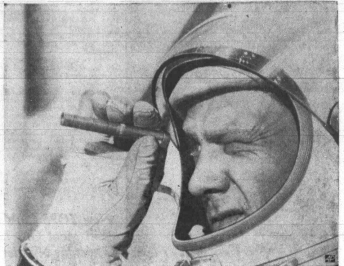
PREP FOR A TRIP — Astronaut Edwin E. Aldrin Jr., peers through a radiation dosimeter during training check for the Gemini 12 orbital mission. Instrument is used inside the spacecraft to measure the ultra-violet radiation during manned missions.
