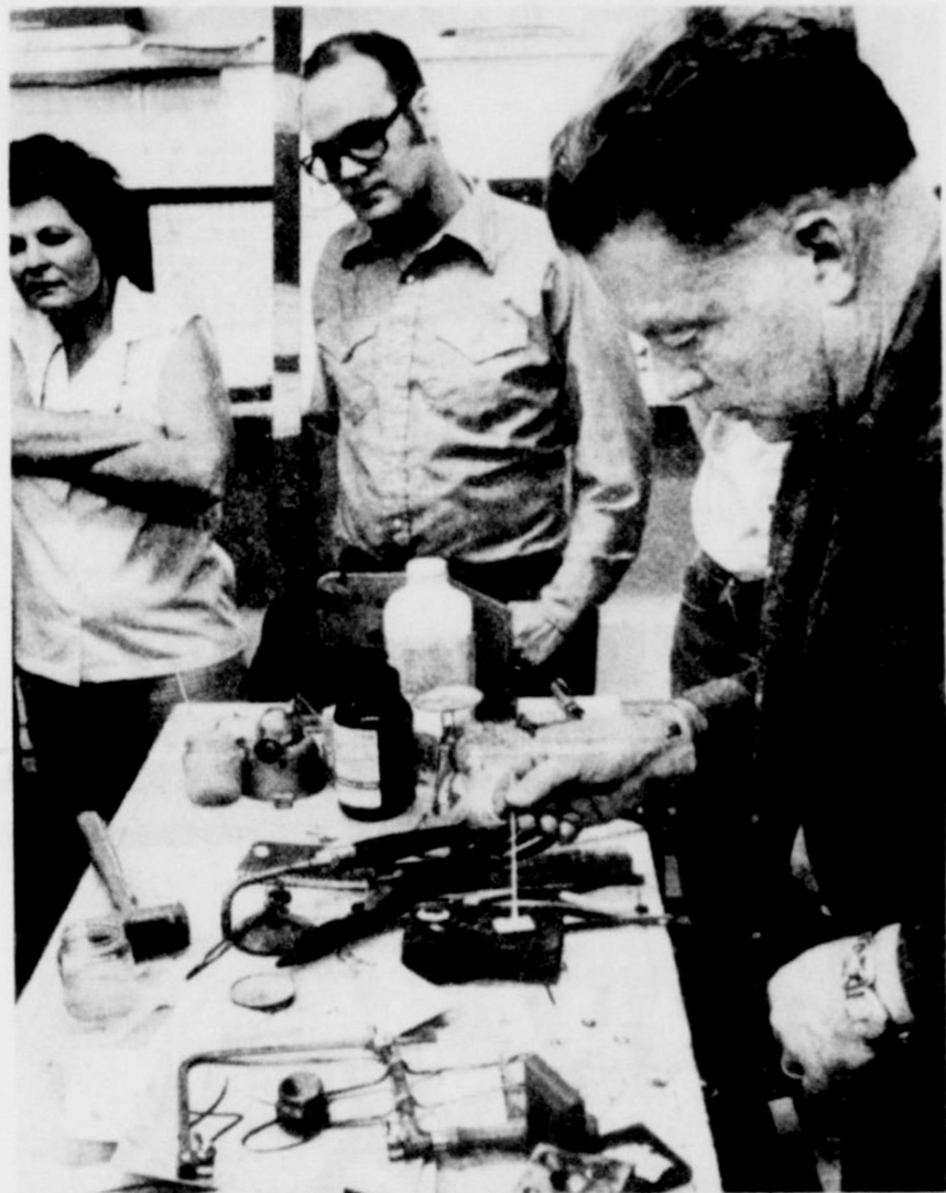
MIKE LAMB and SUE RECTOR watch Leon Coffey apply flux to the beginnings of a shadowbox ring he is making for a class demonstration.
