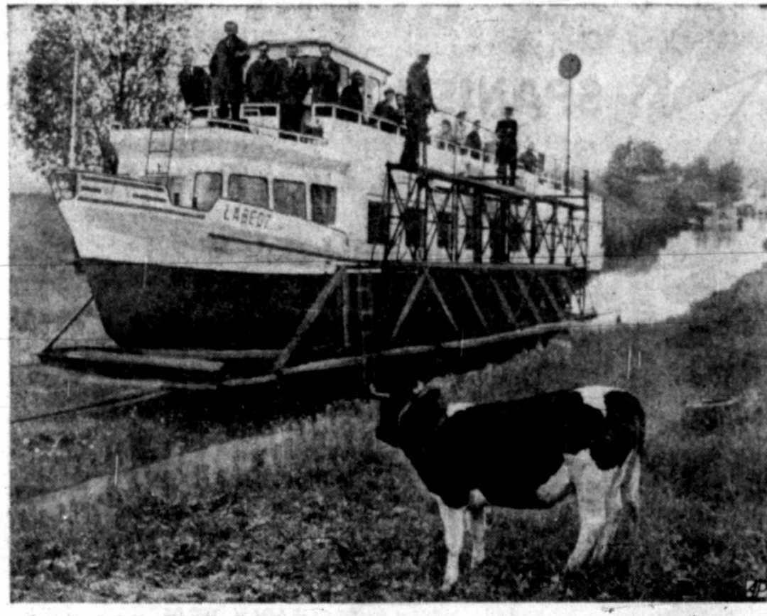
ONE FOR THE BOOK —How often have you seen a boat "sailing" across a meadow? This craft, making its way from Elblag to Ostroda in northern Poland, uses a unique system of rails which enable it to move from lake to lake. The trip crosses 64 lakes.
