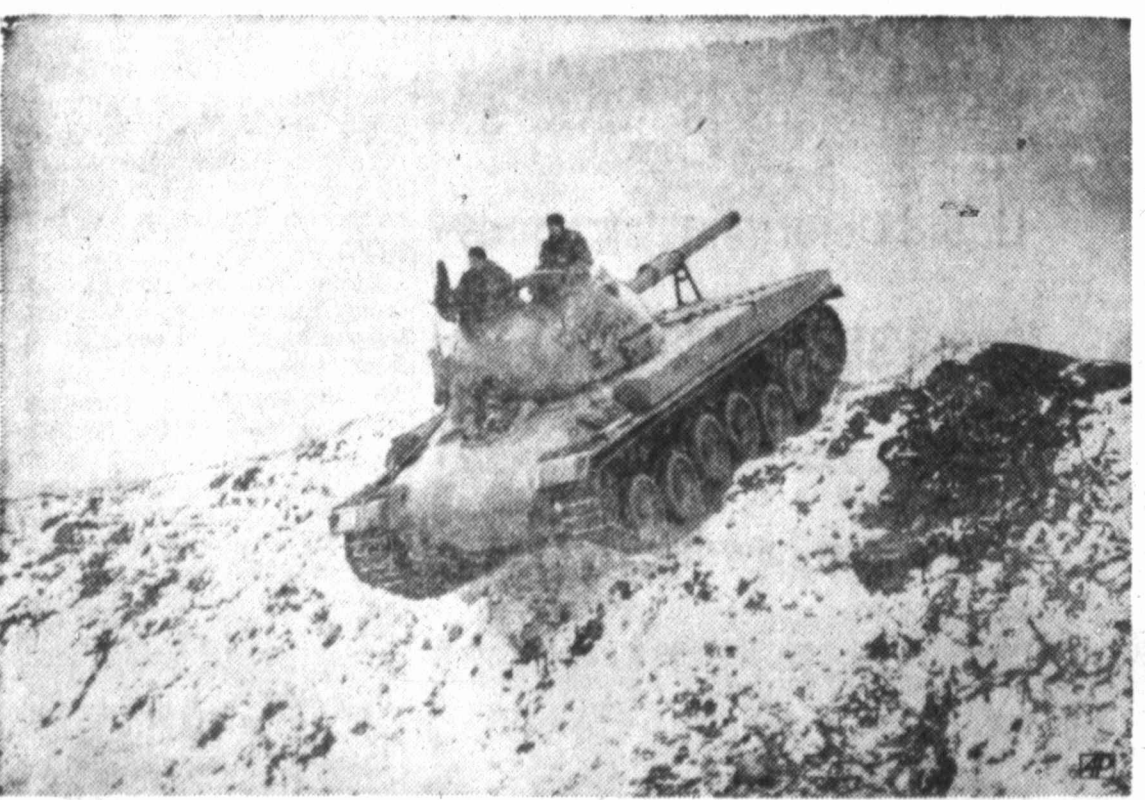
A TEST ON TERRAIN — A new medium tank goes through a demonstration over rough country near Zurich. The four-man, three-weapon vehicle is designed especially for mountainous terrain and the Swiss Army plans to use it chiefly for training purposes.
