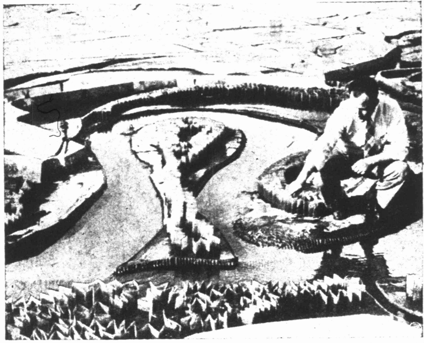
At the 500-acre U. S. Waterway Experiment Station in Vicksburg, Miss., a research worker checks a model site that shows how a bend in the Mississippi River might be cut off to aid navigation and decrease flood dangers. The station has complete miniature scale models of many strategic rivers, harbors and dams, built in 1929 for the scientific study of flood control and navigation.
