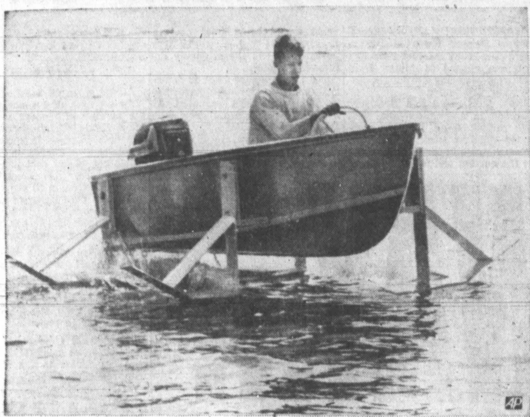
HANDIWORK TEST — Robert Wilkinson, a high school junior, runs his home-made hydrofoil on Seattle's Lake Washington. He uses a 10-horsepower outboard motor which he expects to push his boat to a speed of 40 knots — once the foils are properly adjusted.
