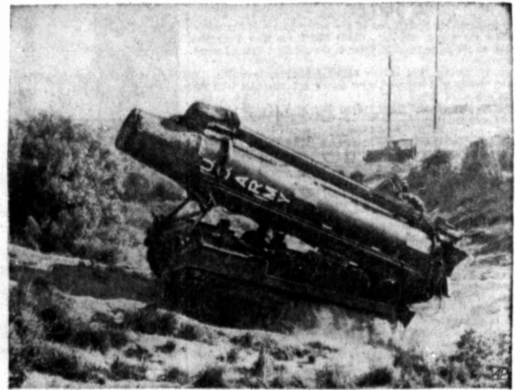
TEST AT THE CAPE —Tracked vehicle transports the Pershing missile through the palmetto and scrub brush at Cape Canaveral, Fla. It was a test simulating rough treatment the Pershing would undergo in combat. Later, the missile was fired successfully.
