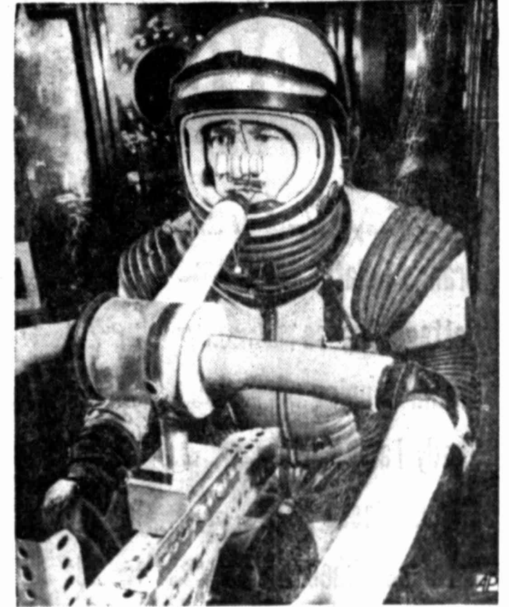
MOON GARB —An engineer undergoes a test in an experimental space suit at Farmingdale, N. Y. The full-pressure suit is designed for the astronauts of Project Apollo.
