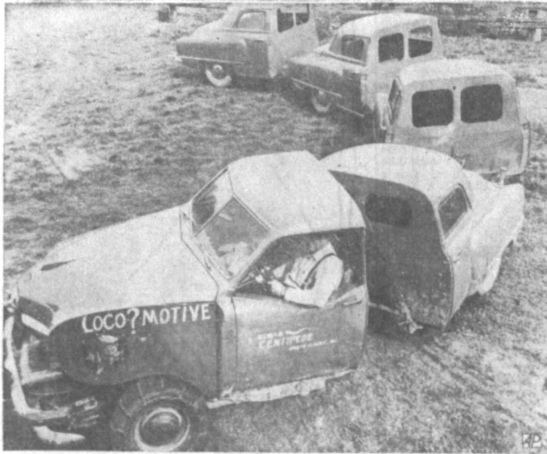
LOCO?-MOTIVE — Elmer and Ervin Wagner of North Plains, Ore., built this auto train by connecting the rear halves of four scrapped cars to the front half of another car which holds the engine. The power is transmitted to the wheels of each unit.
