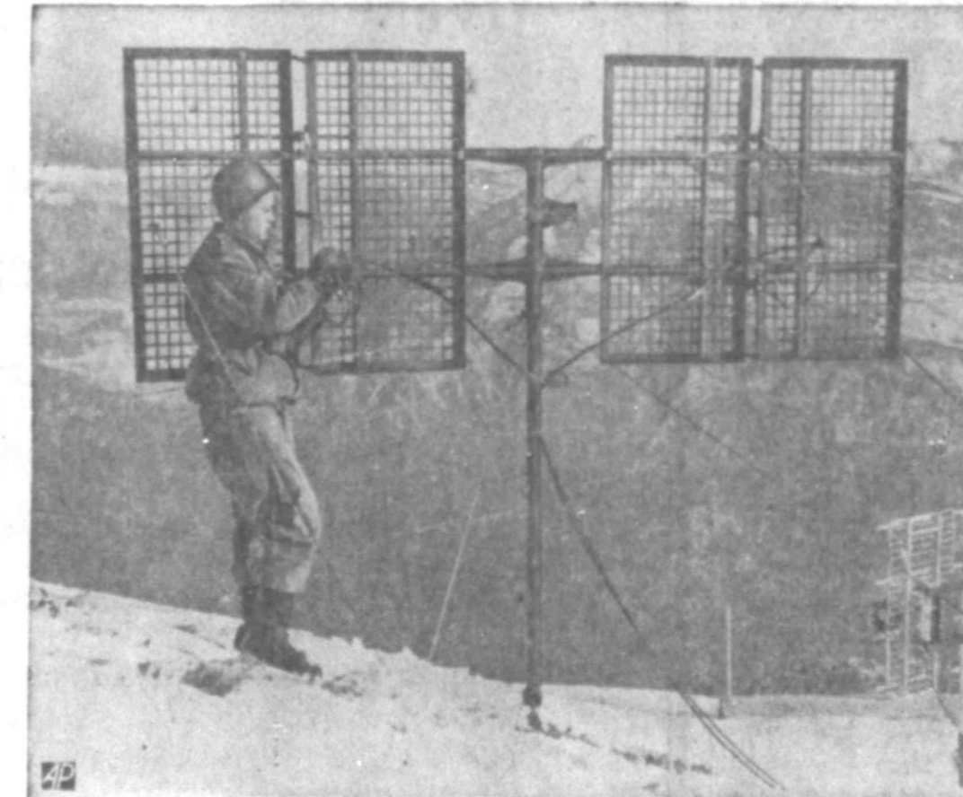
HIGH ON WINDY TOP — PFC L. F. Ferguson repairs UHF antenna atop 6,881-foot Mt. Palon in the Italian Alps near Trento. The station is part of the South European Task Force's vast communications network stretching across northern Italy.
