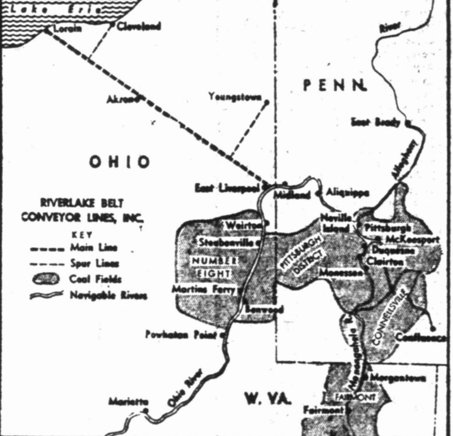
The map shows how the Riverlake lines would cut across Ohio, linking Lake Erie with the Ohio River. The lines will be able to handle 3,400 tons of coal, or 5,400 tons of heavier ore, an hour, and it would take 15 hours and 14 minutes for one ton to go from one terminal to the other.
