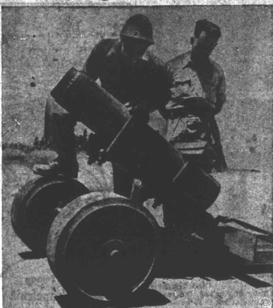
Jewish soldiers look over a home-made eight-inch mortar taken from Arabs during fighting near Tel Aviv. The piece was made by Arab railway workers. To fire a round, they drop a match into a hole in the bottom of the barrel. Job was crude, but it worked. Photo by David S. Boyer. NEA-Acme staff correspondent.
