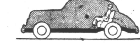
OTHER CARS The car above cannot be streamlined because the need for head room above the rear seat (which is built on top of a frame) makes it impossible to lower the floor.
