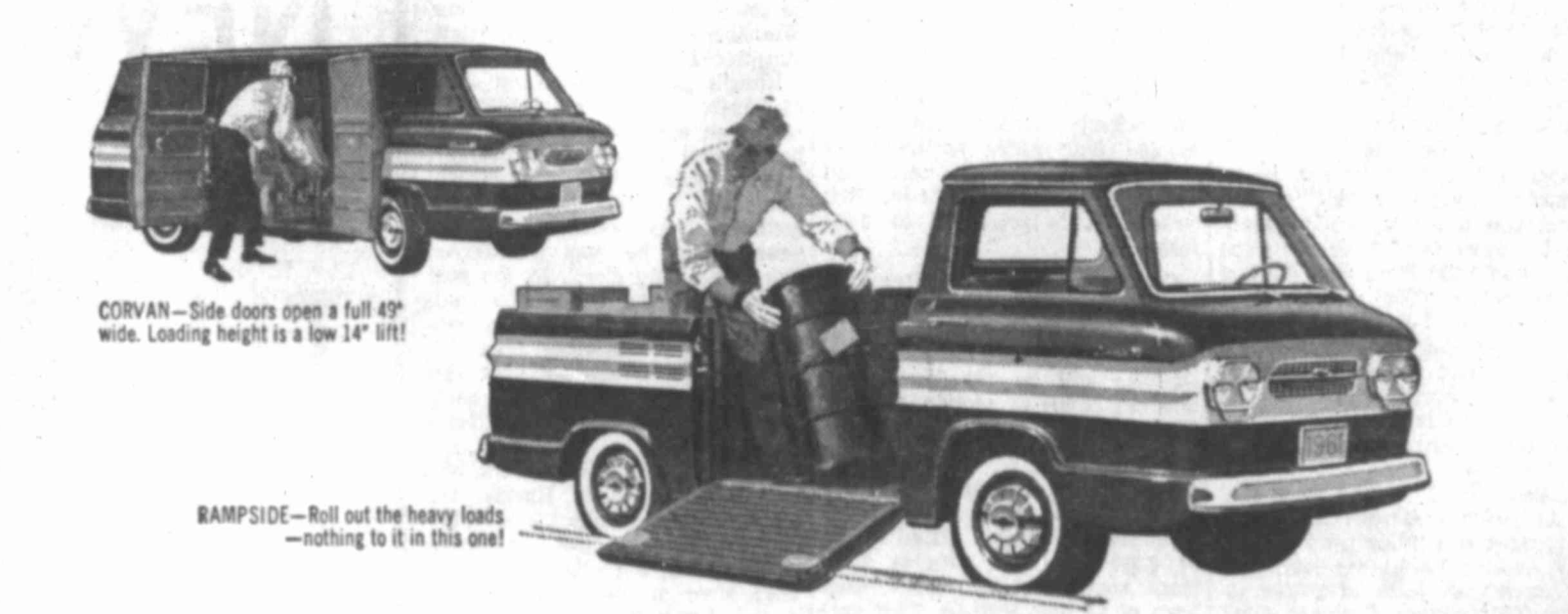
CORVAN—Side doors open a full 45° wide. Loading height is a low 14" lift!
