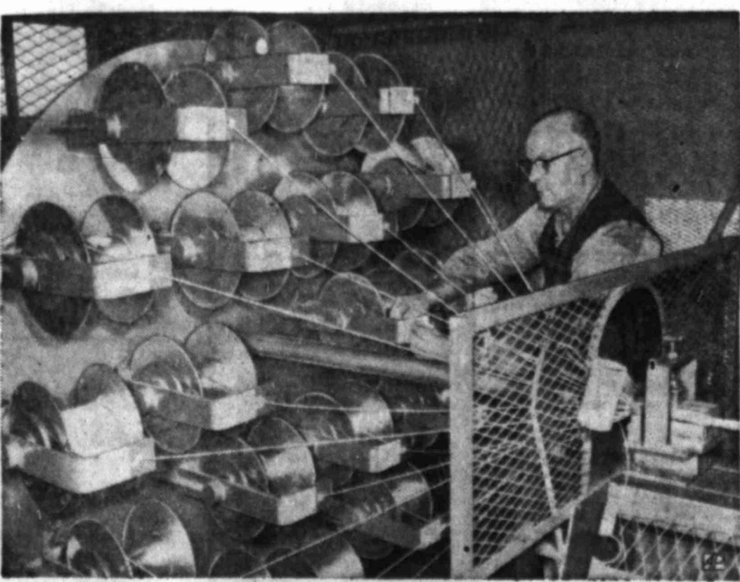
SPACE AGE SPINNER —Technician Arthur Harris checks one of the 18 spools on six-foot diameter wheel of a planetary wire-stranding machine at Van Nuys, Calif. Machine turns out multi-wired cables used for missile and satellite electronic operations.
