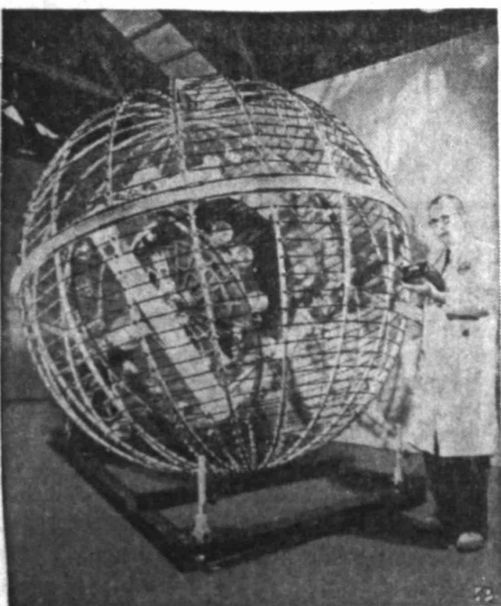
CHECK WEATHER EYE —An engineer checks cage before simulating earth's magnetic field in test of Tiroso II weather satellite of type launched from Cape Canaveral.
