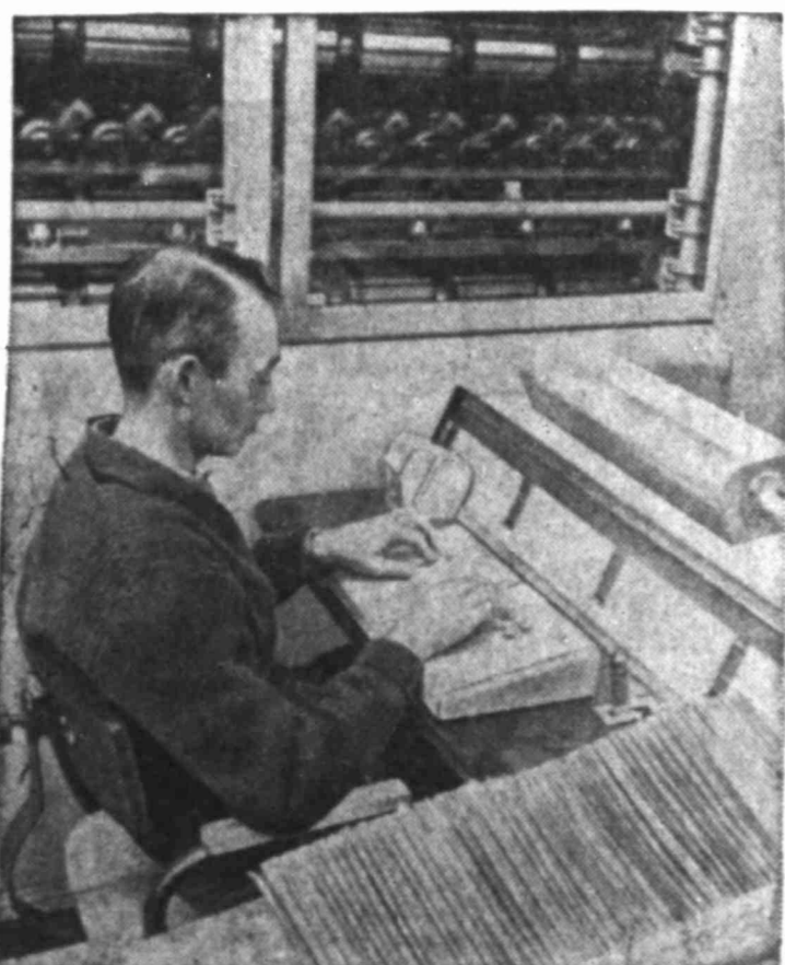
SET FOR SPEED —Clerk scans letter delivered by machine and prepares to punch proper key for sorting in nation's first automatic post office at Providence, R.I.
