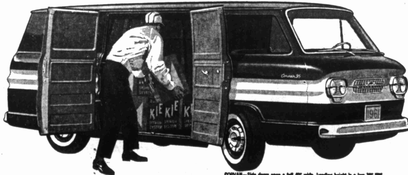
CORVAN —Side doors open a full 48" wide. Loading height is a low 34" high.
